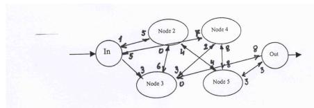
Capacities of roads in terms of the number of vehicles per minute. In WinQSB, select Network Modeling. In Problem Type, select Maximal Flow Problem. The Objective Criterion is by default Maximization.
