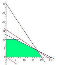
The solutions  $x_1 = 17.5$ ,  $x_2 = 3.75$  are not integers. Thus we have to find the point(s) in the green area which have integer coordinates and for which the value of  $z = 20x_1 + 30x_2$  is the largest. This point is  $x_1 = 17$ ,  $x_2 = 4$ , and  $z_{max} = 460$ .
